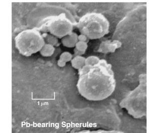
**Fig. 5.** Scanning electron micrograph of clustered, spherical leaf particulates, Grapes Hill, Norwich. From EDXA analysis, Pb occurs (as a minor element) only within the spherules <1 μm diameter.
