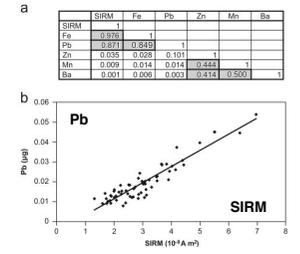
**Fig. 3.** Correlations between leaf particulate metal concentrations and SIRM, Grapes Hill, Norwich: (a) all analysed metals ( $n=40$ ), shaded boxes with significance  $<0.05$  and (b) Pb concentration and SIRM ( $n=40$ ,  $p<0.0005$ ).
