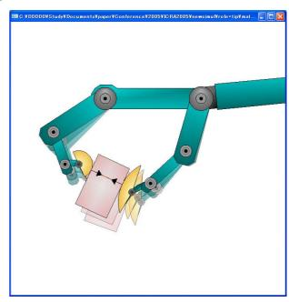
Robotic grasping on the basis of pad-opposition of thumb and index finger
