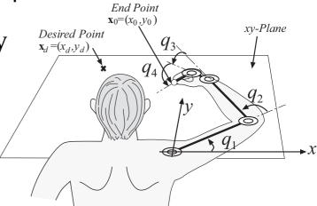
Multi-joint point-to-point movement with redundant DOFs.
