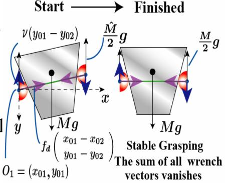
Blind Grasping without knowing object kinematics, without using any external sensing
